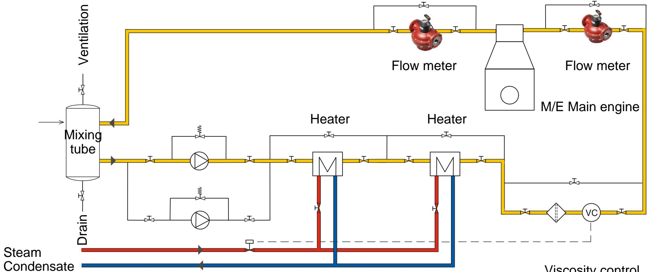
Flow measurement in the circulation after mixing tube
